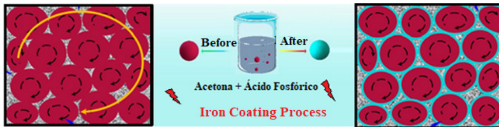
Figure 6: Schematic diagram of the eddy current loss reduced by the effectively integrated insulation coating layer
